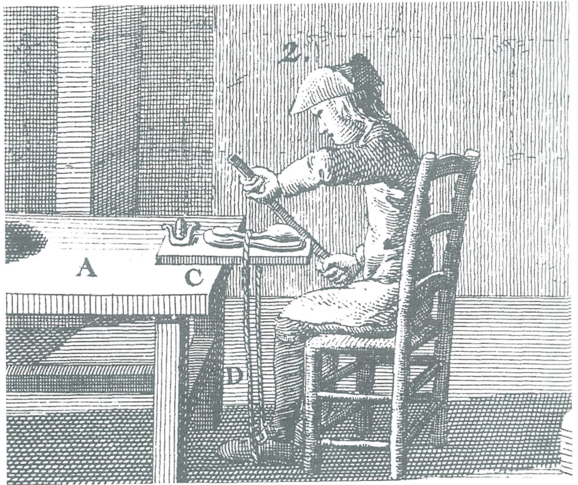
3. Detail from Pl. 4 of L'Art du potier en terre . Master pewterers or neymen skimmed or smoothed pewter objects by holding a tool and a hook against them as they turned on a lathe turned by a helper.
