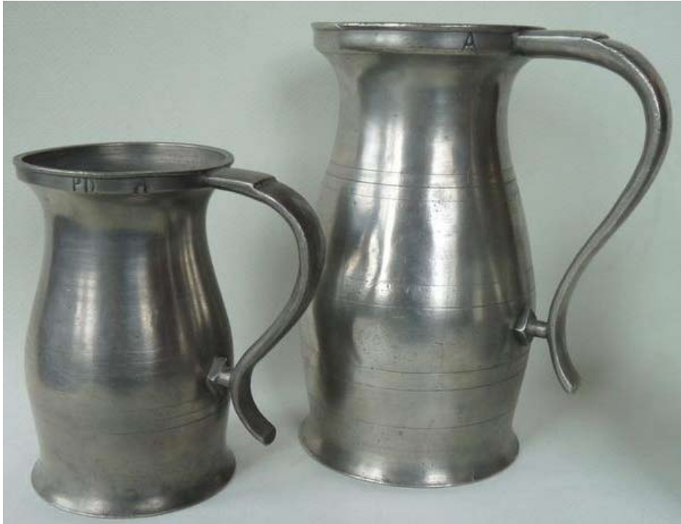
Figure 12. Pint “A” also verified for as a Vermont town standard, together with an “A” quart of similar type. Pint: height to brim 5 \frac{1}{8} ”, top diameter 3 \frac{3}{16} ”, base diameter 3 \frac{1}{4} ” Quart: height to brim 7”, top diameter 3 \frac{3}{4} ”, base diameter 3 \frac{7}{8} ”
