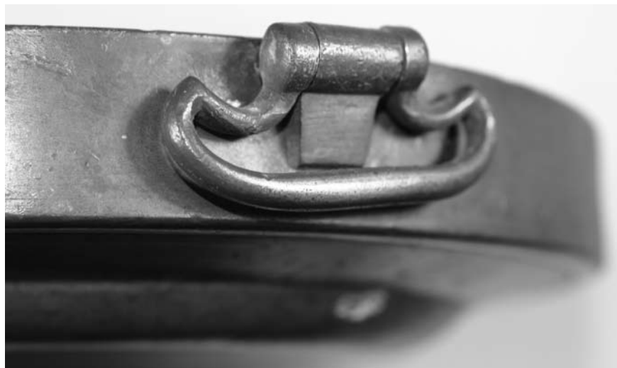
Fig. 3. Handle and hinge attachment on Byles water plate.
