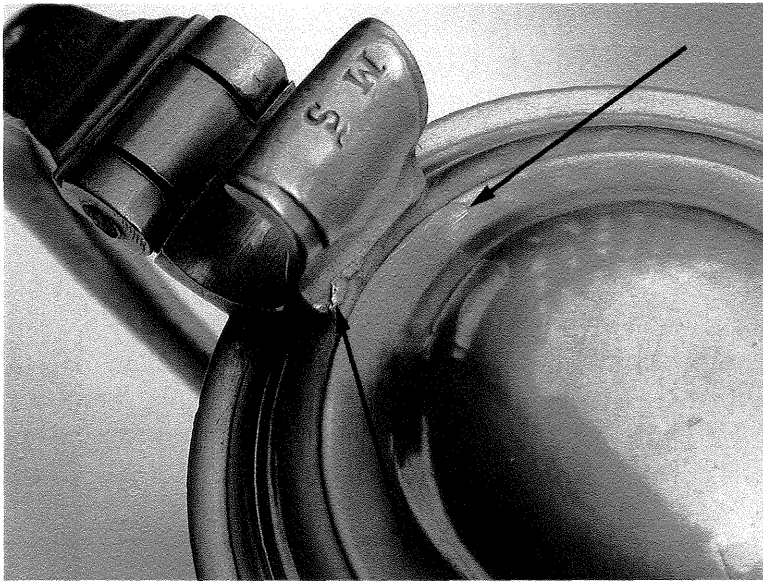
Fig. 2 .Left arrow shows excess solder that didn't melt fully nearest to left side of thumbpiece. Arrow to right shows overflow of solder.
