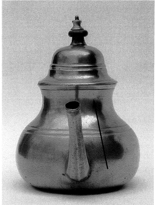
Fig. 26. Note the angle of the spout leaning to the left. Spouts and handles were not always put on as straight as they could be.
