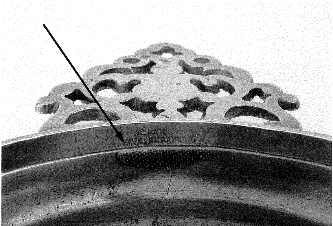
Fig. 7. The arrow shows a typical “linen mark”. This is the result of molten metal flowing into the handle mold melting through the body casting and being dammed by the linen “tinker’s dam” on the inside of the porringer bowl.
