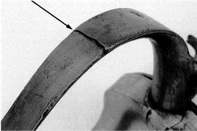
Fig. 19. Note the “crack” in the handle on this half-gallon bud baluster measure. This was caused when the linen tinker’s dam was removed too soon. The metal had not completely solidified and moved slightly forming this crack.
