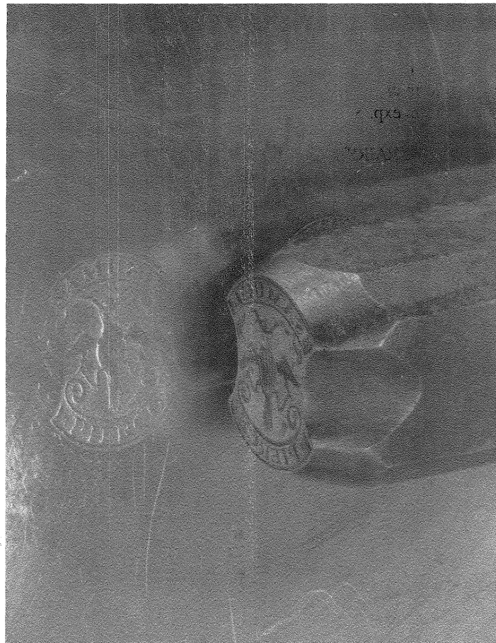
Fig. 1. Die, attributed to Samuel Pierce, Middletown, CT., or Greenfield, MA., late 18th-century. Steel; L: 6", Diam.: 1 1/8". Courtesy, Historic Deerfield, Inc., gift of Ledlie I. Laughlin. Photography by Penny Leveritt unless otherwise cited. This die is the only known surviving touchmark of an American pewterer.
