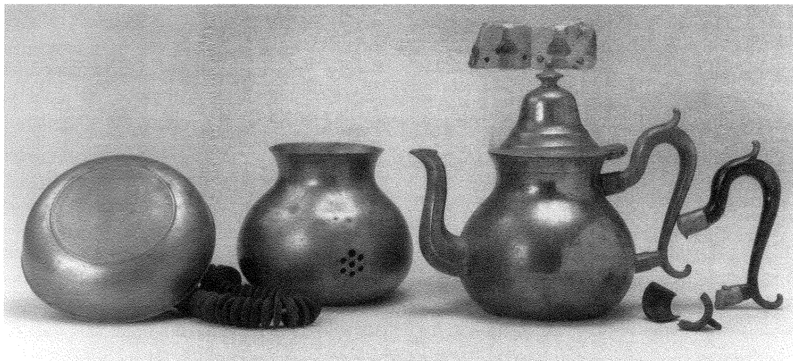
Fig. 8. Teapot, Teapot Parts, and Molds by Samuel Pierce, Greenfield, early nineteenth-century. Pewter, soapstone, brass. Teapot H: 7", W: 8 1/2" with spout and handle, D: 5 1/2". Historic Deerfield, Inc.; gift of Ledlie I. Laughlin. Pierce cast and assembled his teapots from about a dozen components, some of which have survived as scraps along with the molds that made them. At the top is the soapstone mold for the finial; at the lower right is the small bronze mold for the ferrule that secures the lower end of the handle.
