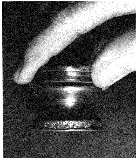
Fig. 2. Hand-held approximate quarter-gill measure of the bulbous form showing some of the many plain "X" marks stamped on the measure's collar cancelling numerous verifications seals and indicating that the measure no longer complies with the legal standard capacity. Courtesy of Ian D. Robinson.
