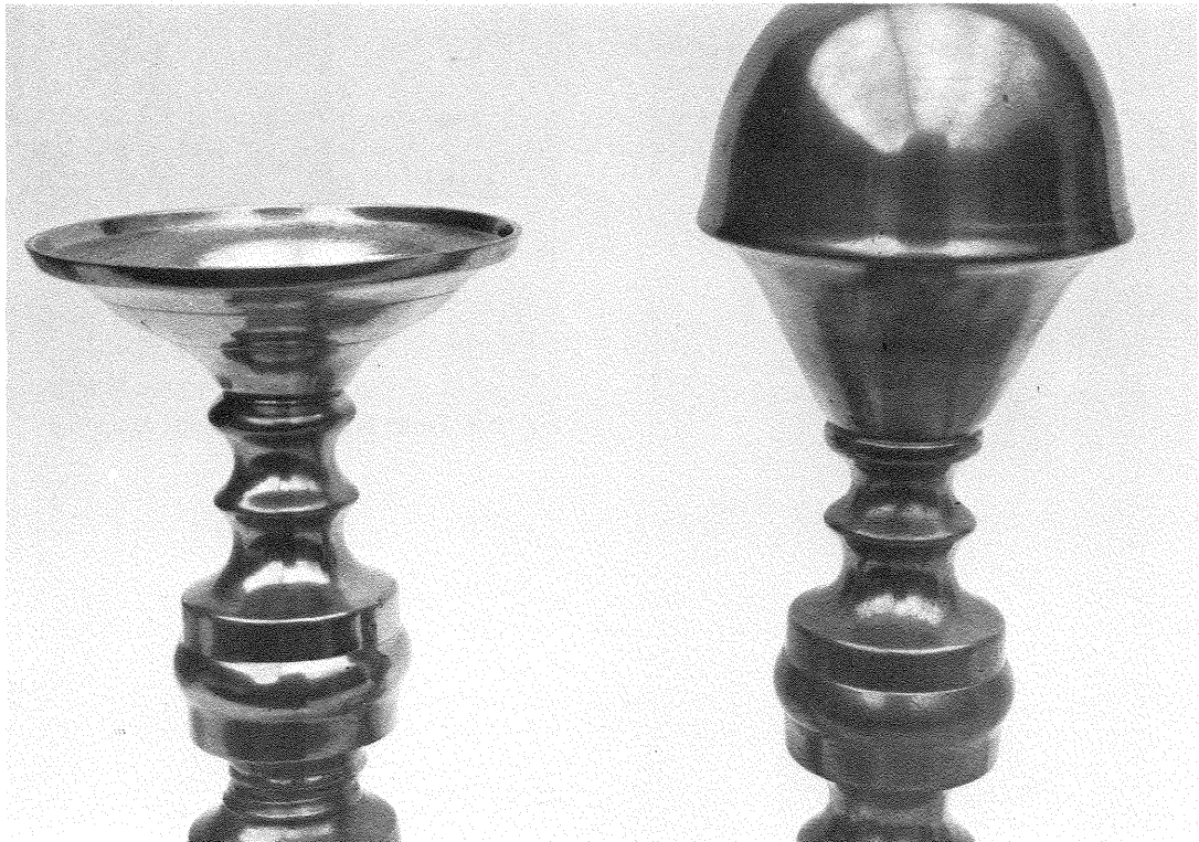
Fig. 27. Interchangeability of parts on Porter pieces
