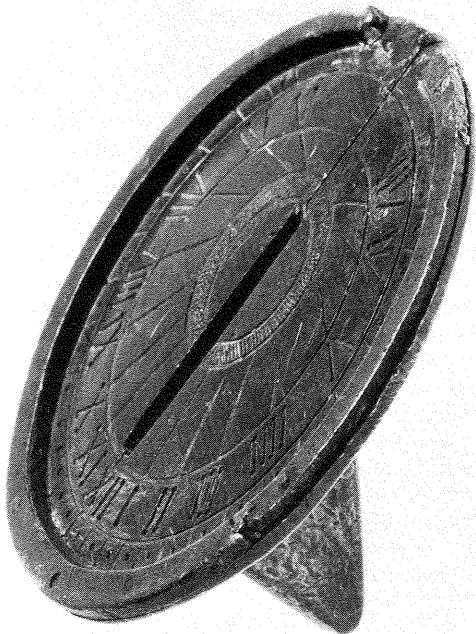
Fig. 2 — Mould for making 4 1/2" pewter sun-dials. Private collection.
