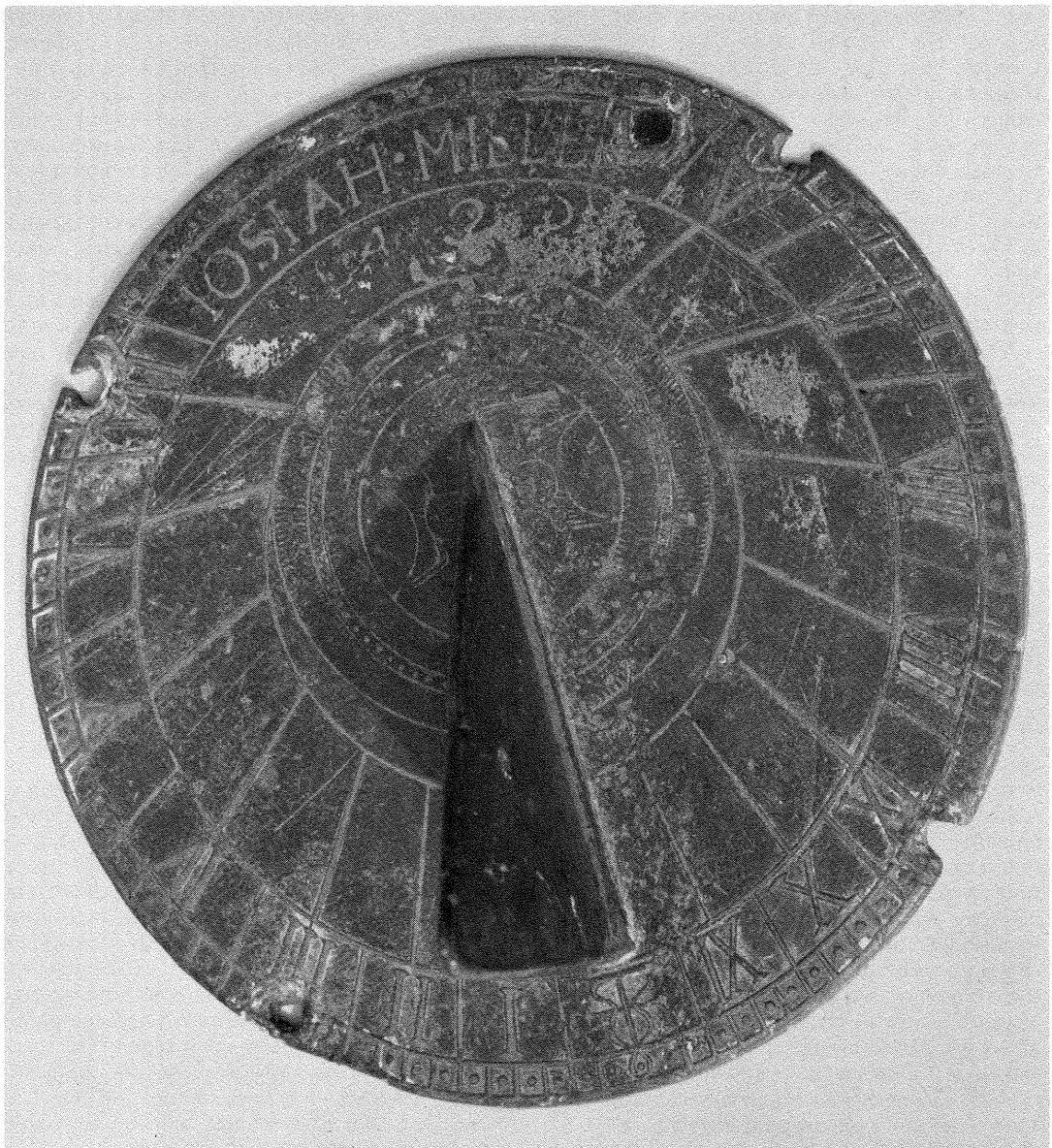
Fig. 6 — Pewter sun-dial from the Josiah Miller mould illustrated in Fig. 2. Dial is at the Leffingwell Inn in Norwich, Conn. Courtesy of the Society of the Founders of Norwich, Conn.
