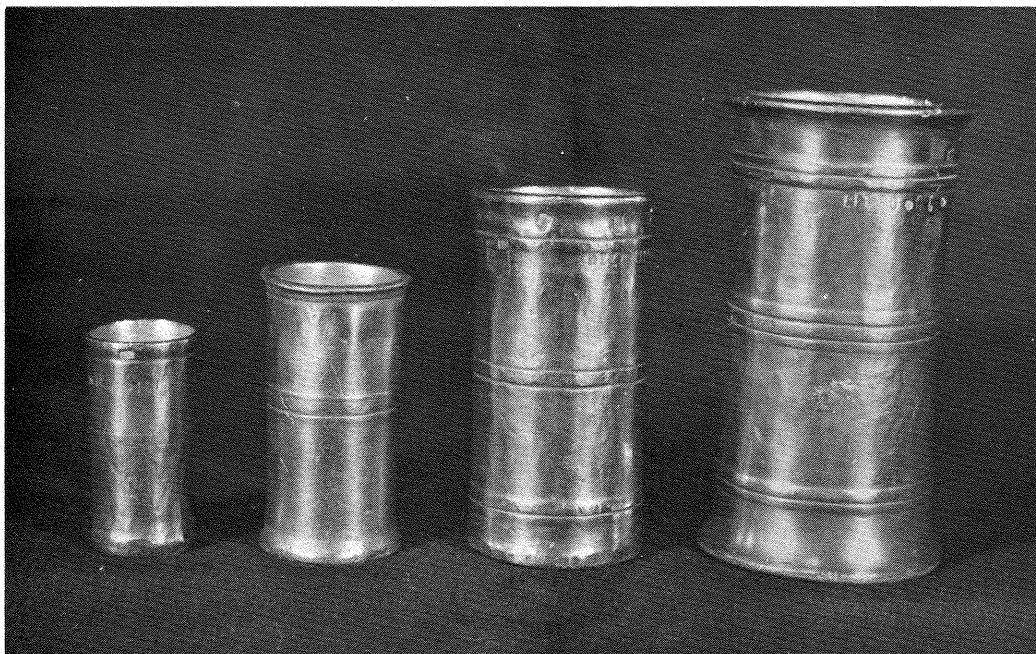
FIG. 1. Italian Metric Measures of (l. to r.) Decilitro, Doppio Decilitro, Mezzo Litro and Litro capacities.
